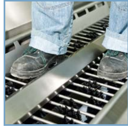
Aktive Reinigung durch rotierende Bürsten Active cleaning with rotating brushes
