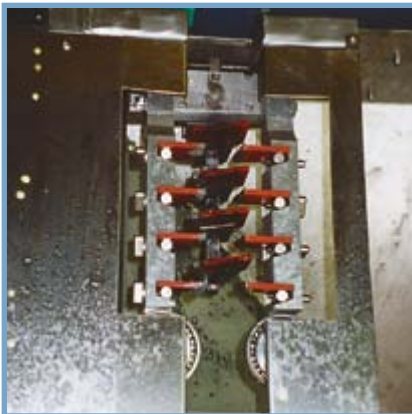
„Mitfahrende“ Abziehvorrückung Wipers carried along with the skid
